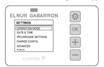
Use or to move up and down. Confirm with to enter the desired setting.
