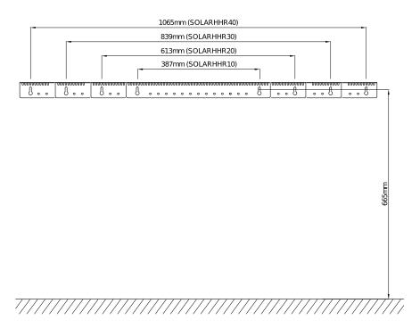
5.- Fix the side fixing plates to the metal casing by using the appropriate screws. The supply cables must be fitted but not wired to the storage heater before placing the heater to the wall. Remove the white screws located in the top of SOLAR HHR, and place the SOLAR HHR in the selected installation area. Use the removed screws to attach SOLAR HHR to the top fixing plate installed in the wall.
