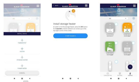
When required, keep pressed button during 3 seconds until the symbol is displayed in the storage heater display.
