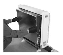
9.- Do not disconnect the electrical heating elements. Remove the packing cardboard and the metallic plate. Lift and tilt the elements outwards being careful not to damage the insulation on the bottom of the heater and carefully place the storage bricks. Arrange two levels of bricks with the flat side facing to the back of the heater.
